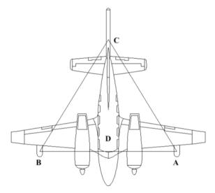
Figure 3 – The GRAVEX configuration on the aircraft. Each wing pod and the stinger carry a single miniature, temperature and axis-stabilised gravity sensor (ABC), together with one at the aircraft centre of gravity (D), acting as a reference. Typical dimensions of the gradient triangle formed is 10 metres per side.
